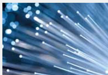
is used for optical data transmission. Compared with traditional means via copper cable, it offers a far higher maximum bandwidth. Optical fibers are also insensitive to electrical and magnetic interference fields and offer higher immunity to tapping.
